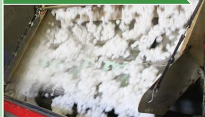
The modules are taken to the cotton gin where the cotton will be dried, cleaned, and have its seed and fiber mechanically separated. The gin contains revolving circular saws that pull the raw fiber through closely-spaced ribs that prevent the seed from passing through.
